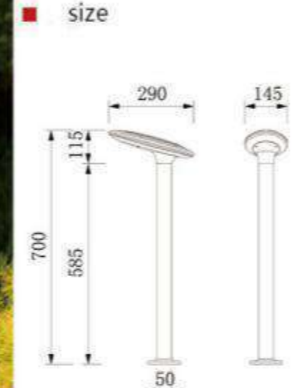
Model: Star light lawn lamp Light source type: LED Power: 5W-10W Size: L290*W145*H700 Material: Die-cast aluminum Voltage: < 36W or = 36W Protection grade: IP65
